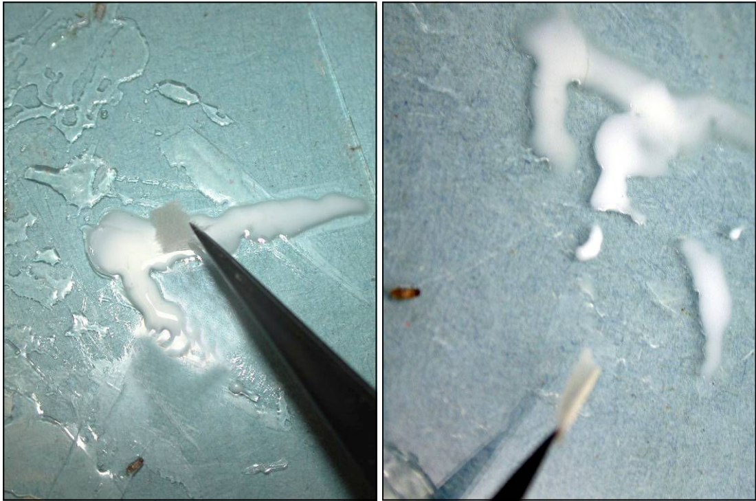
Fig. 4. Dragging the tissue strip through the glue and way out the other side will prevent it from rolling up (right) – note the glue trails (left & right).
