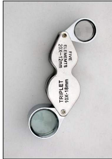
Fig 2. Triplet magnifier from United Kingdom Geologists Equipment (UKGE) provides a choice of two lenses: x10 and x20, the lenses being 18 mm and 12 mm diameter respectively.
