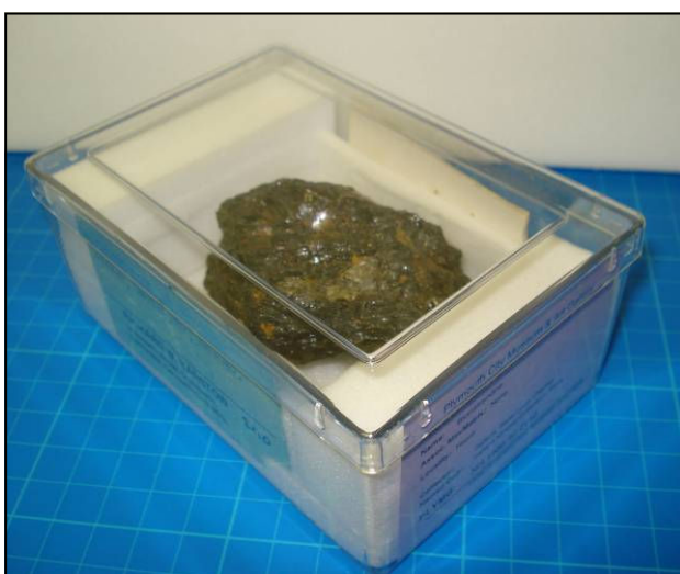
Fig. 1. Torbernite specimen re-packed in clear polystyrene plastic container, with Plastazote lining. The associated labels are facing outwards to minimise any disturbance of the specimen.
