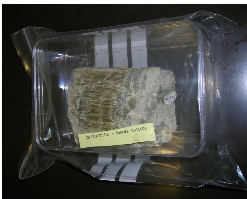
Fig. 3. Chrysotile specimen stored in clear box in zip lock bag. This method was suitable for the funds available at the time, and the storage will be reviewed in the future.
