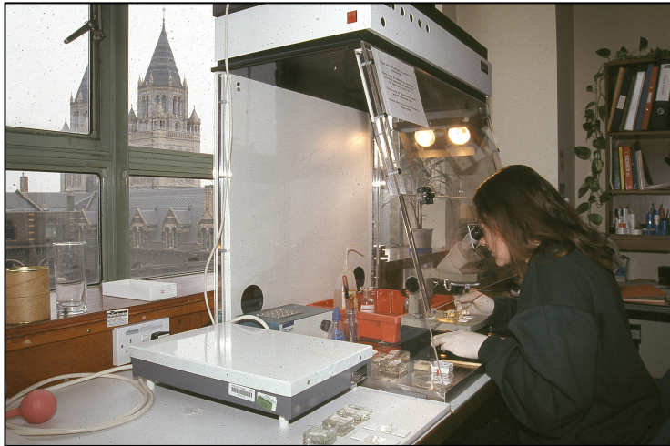
Fig.1 Hazardous chemicals such as glacial acetic acid, phenol and xylene require the use of a portable fume hood.
