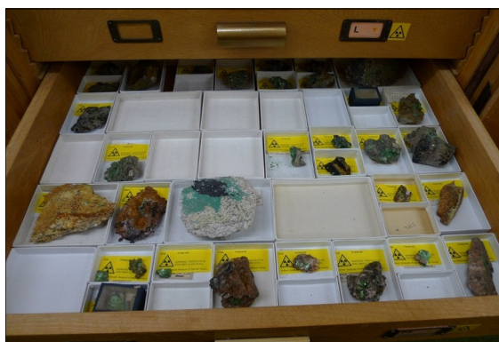
Fig 6. 'Low level' radioactive minerals at Oxford, for which both drawers and individual specimens have yellow radioactive warning labels. (photo: Oxford University Museum of Natural History)
