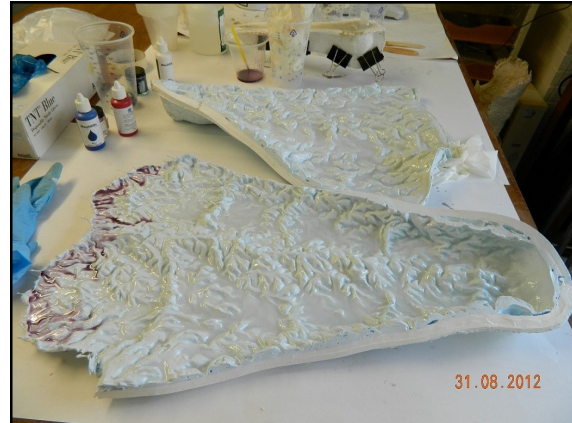
Fig. 10. Filling the two part silicone moulds of the oral arm with polyester resin.
