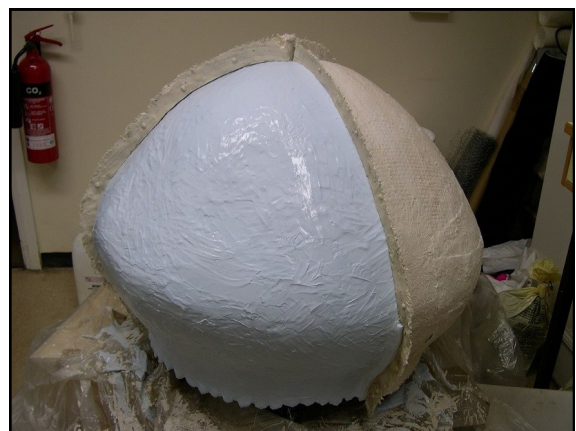
Fig. 5. One part silicone mould and three part Jesmonite support case. Holes were drilled into the edges to bolt the sections together.
