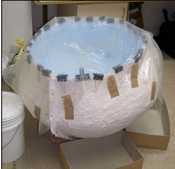
Fig. 9. The completed jellyfish bell mould ready for heating prior to casting with Polyoptic resin.
