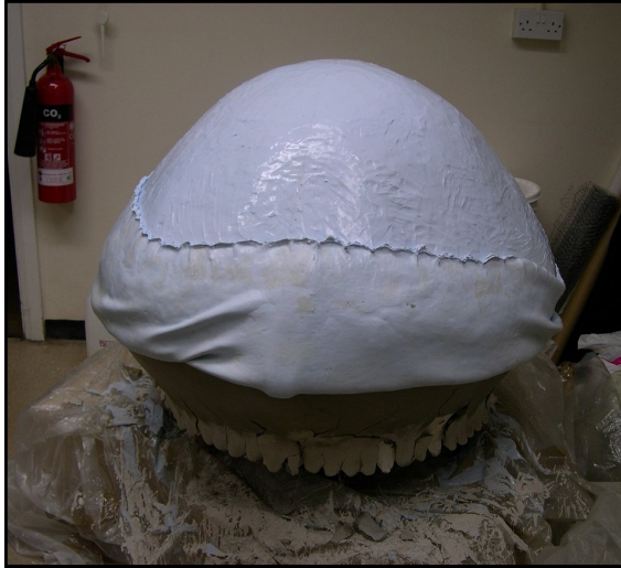
Fig. 6. The cured single piece silicone mould being peeled off of the wet clay sculpture.
