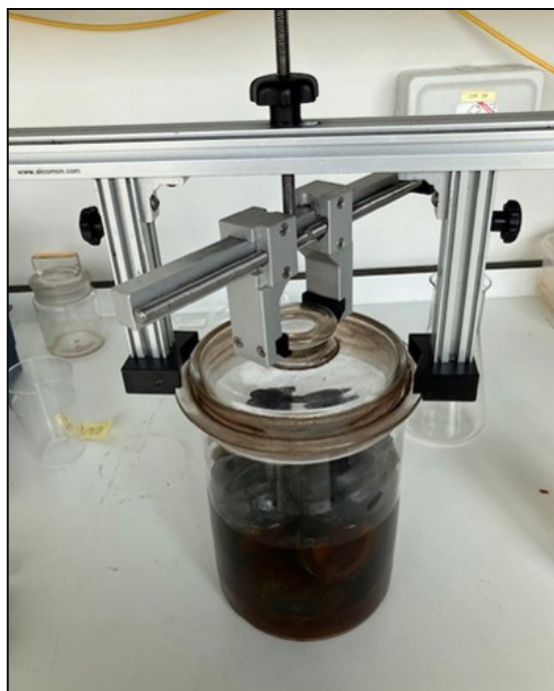
Fig. 8. Universal stopper jar opener designed by Andries J. van Dam in collaboration with the Natural History Museum, London.
