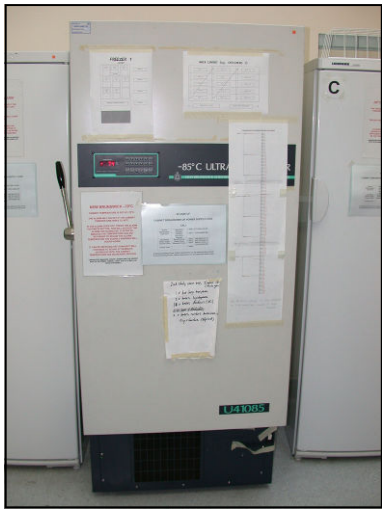
Plate X. A -80^{\circ}\text{C} (or ultra-low) freezer in the Entomology Department Molecular Laboratory, The Natural History Museum, London
