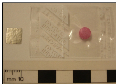
Fig.3 Oxygen indicators: on the left is a SensiSpot™ and on the right an "ageless eye".
