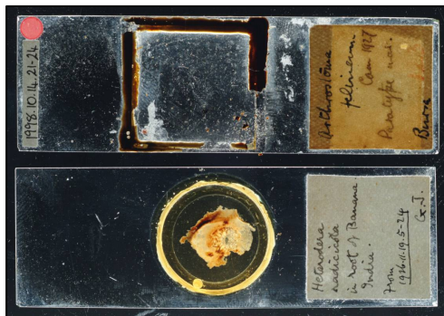
Fig. 1 A - Sealant has become brittle and chipped away leaving the mountant exposed. B - A reaction has occurred within the slide. Possible cause oxidation, indicating the slides sealant has been breached.
