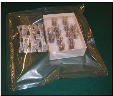
Fig. 4 Glass vials sealed with 13 sealants, plus one control, each with a SensiSpot on inert foam. The tray is in a microenvironment created with
