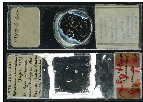
Fig. 2 A - Sealant breakdown evident as air has entered the slide, also possible reaction between mountant and sealant evident. B - Wax sealant has broken down. A reaction in the bottom corner is also now evident, if this were to continue it could cover the slide obscuring the specimen.
