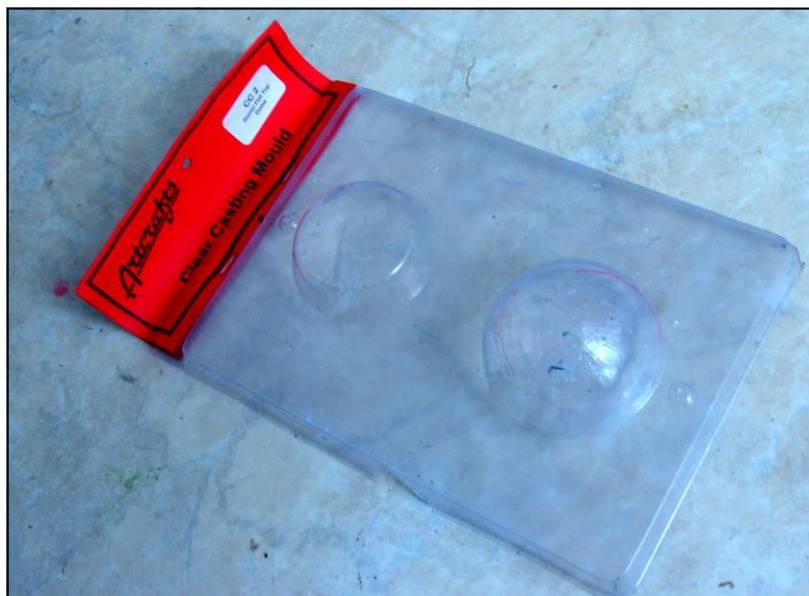
Fig 2: A clear polypropylene casting mould.
