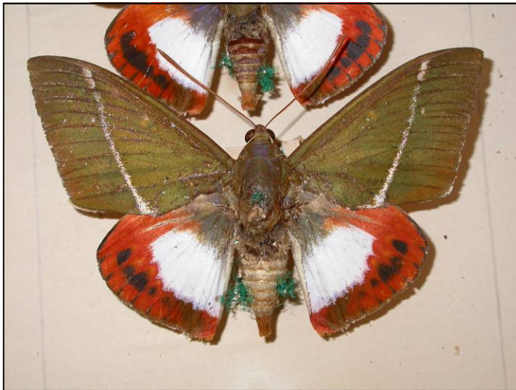
Fig. 4. Verdigris formation on a non-stainless steel pin and cross-pins around a castniid moth.
