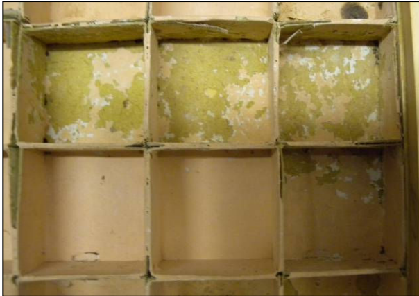
Fig. 3. Fungal and insect damage to paper and card compartments.
