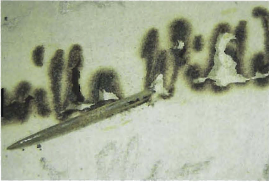
Plate 37 Example of an early acidic 'iron gall' ink which has eaten through the paper (reproduced with kind permission from the National Museums and Galleries on Merseyside).
